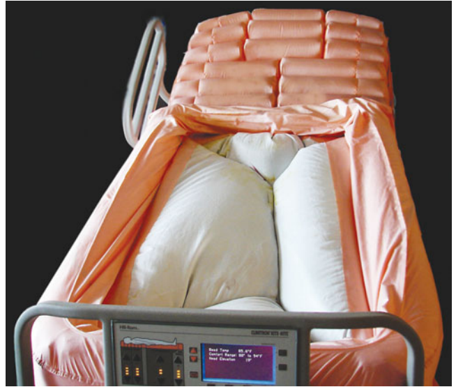
Figure 2-4. Specialty pressure relief air/fluid mattress, in which warmed air passes continuously through beads and the mattress surface, minimizing local skin pressure.
