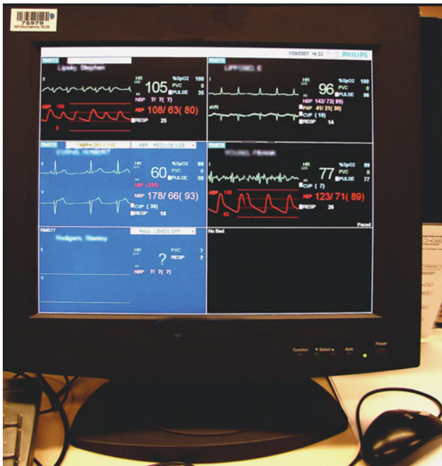
Figure 1-3. Central monitor on a nursing unit, where the key data from all of the patients on a unit are aggregated, and from which alarms are generated to all providers on a unit.
