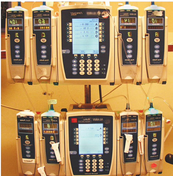
Figure 1-14. Infusion pumps, used to control the rate of delivery of fluids or medications to a patient, and prevent infusion of air or debris.
